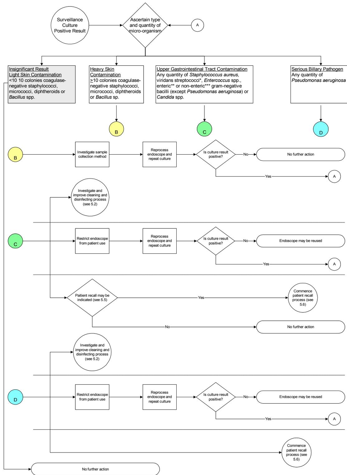
The horizontal broken lines in each process separate pathways that must each be followed
